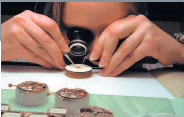
Hard at work in the Caliber 5011's final assembly atelier, watchmaker Julia Viecenz scrutinizes the Nivarox 1 balance-spring with its characteristic Breguet curvature.
