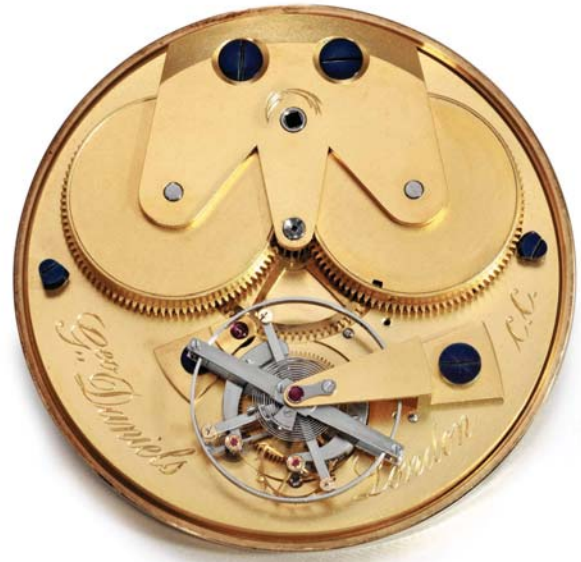
The Daniels Pocket Watch with pivoted detent tourbillon carriage. Image courtesy of Sothebys.
